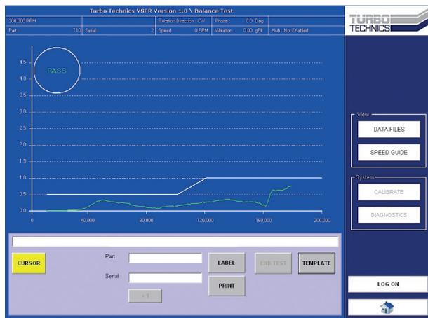
Easy to use computer interface, with visual vibration graph, allowing identification of imbalance.
